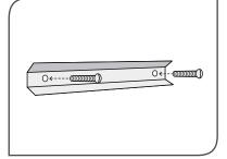
STEP 4 – Attach the mounting bracket to a secure vertical wall, making sure to keep it level. (Screws not included.) (Total weight with plants is approximately 25 lbs.)
