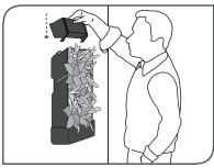
STEP 6 – Slide the GroVert Irrigator into the top planter grooves for easy watering.
