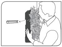
STEP 5 – Simply set the GroVert planter onto the secured wall bracket by matching the notch in the planter back over the bracket.
